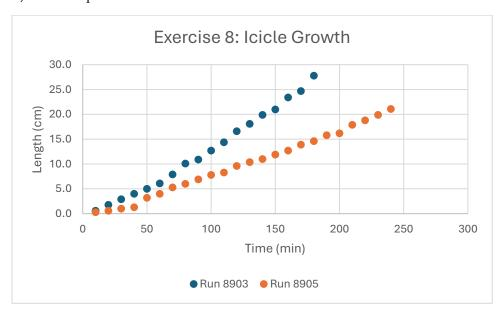
b) Both runs show an increase in length over time. Run 8905 had a higher water flow but a slower growth than run 8903, resulting in shorter icicles, whereas run 8903 produced longer icicles. It means that higher flow makes the water more difficult to freeze.
